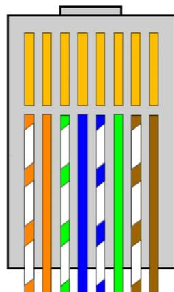
Ensure that the copper ends are all flush with the end of the RJ-45 connector before crimping it
